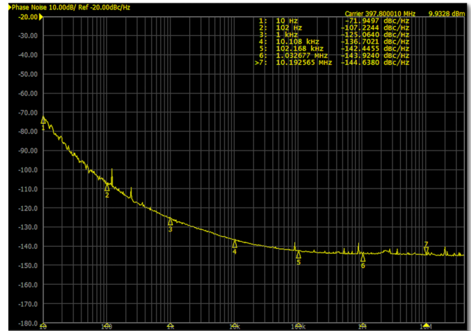
Phase Noise: 139 dBm/Hz, 20 kHz Offset; Fc= 398.7 MHz, +10 dBm (1 GHz TCXO Option 020)
