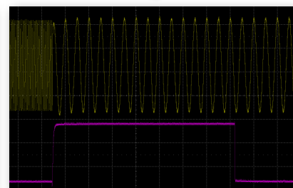
Sweep-Frequency Start Sync 15 \mu s Pulse EXT Free Run (Trigger Out)
